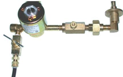
**Do not use Teflon thread seal tape when installing this device. If sealing of threads is required, use a pipe joint compound (pipe dope).**
